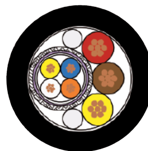
Structure Hybrid cable
